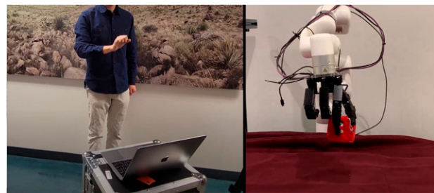
Figure 2. An operator completing a dice pickup task while watching the robot through a video conference. Video demos are at https://robotic-telekinesis.github.io/ .
