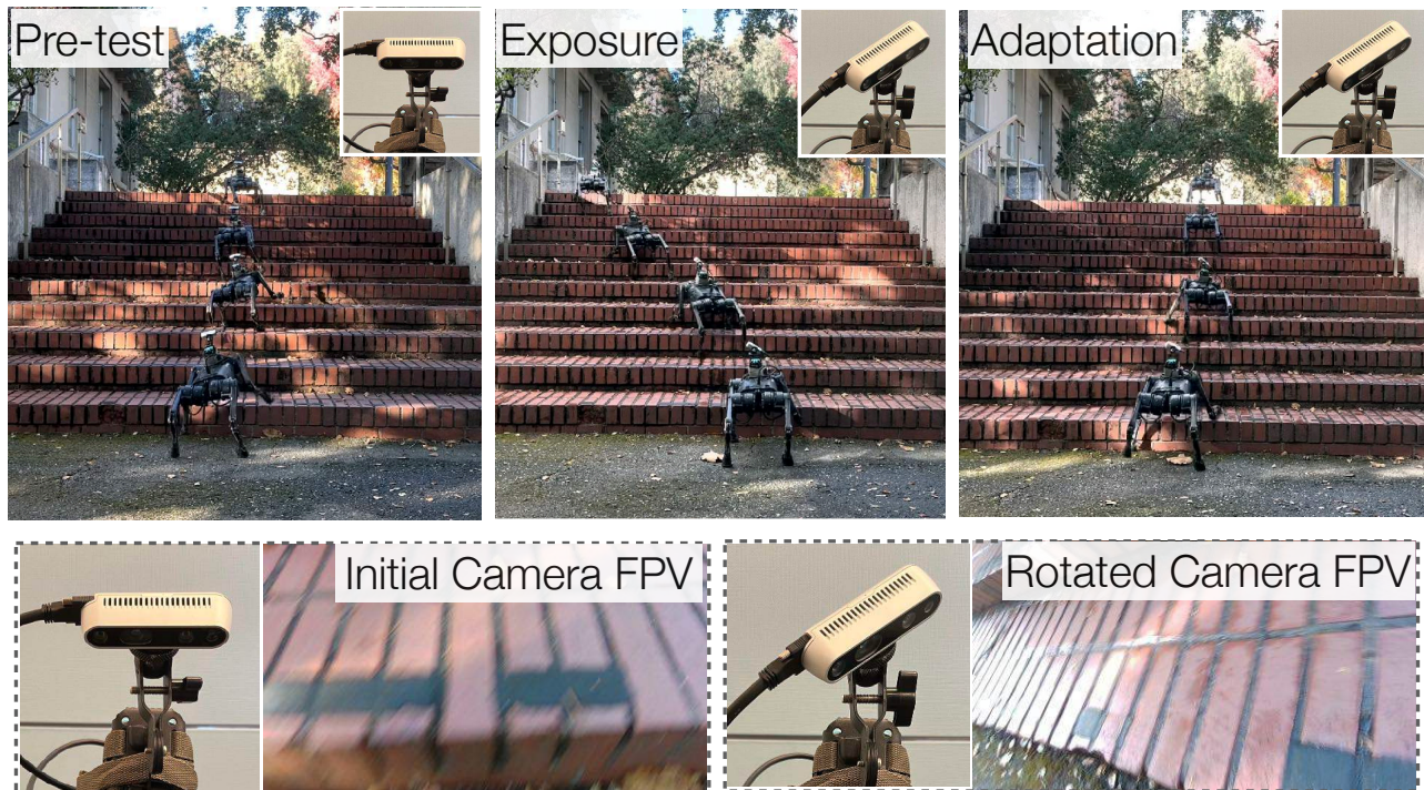
Fig. 5: Prism-Adaptation Test: We perform the widely-known prism test [16] on our robot. In this test, the visual field of the subject is altered by using a prism in front of the eyes. To simulate this, we rotate the camera from its nominal position, and then the robot attempts to perform the task with a visually different input. (Top Row) The left image shows the visual walking policy under nominal conditions, the center image is the performance of this visual walking policy immediately after the camera is rotated, and the right image shows the performance after training for 80 seconds of experience. We can see that the behavior recovers with just 1 minute of finetuning on the new visual input. (Bottom Row) The left camera is the nominal position, and the right camera is the one after rotation. The view from the camera is shown next to the camera orientation. Note the drastic visual change between the two images.
