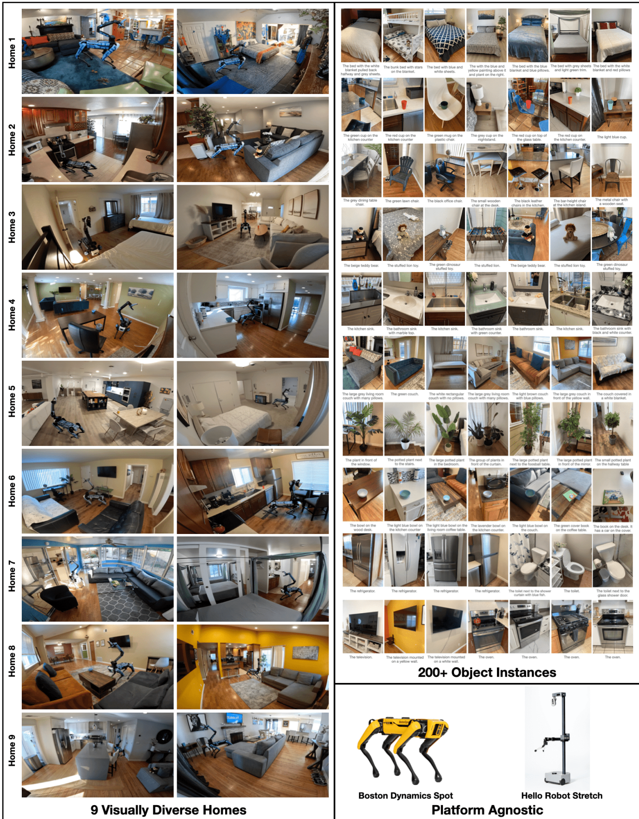
Fig. 5. “In-the-wild” evaluation. We deploy the GOAT navigation policy in 9 visually diverse homes and evaluate in on reaching 200+ different object instances as category, image, or language goals. GOAT is platform-agnostic: we deploy it on both Boston Dynamics Spot and Hello Robot Stretch.
